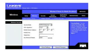
Figure 8-23: Wireless Tab - Wireless Security (WPA Enterprise - TKIP)
